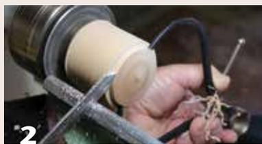
**1** Measure the inside diameter of your espresso maker's filter basket, then turn the tamper to that size. Use a close-grain hardwood for this part of the project.
