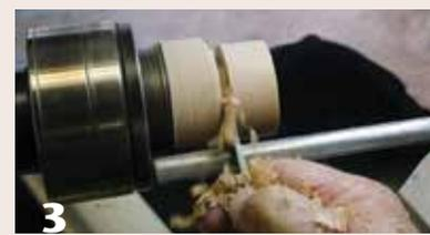
**3** The author uses a parting tool to turn a tenon and shoulder on the tamper.
