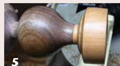
**5** Rough-shape a contrasting species for the knob, then drill a hole to accept the tenon on the tamper. Glue the sections together, turn a smooth transition, and finish shaping the knob.
